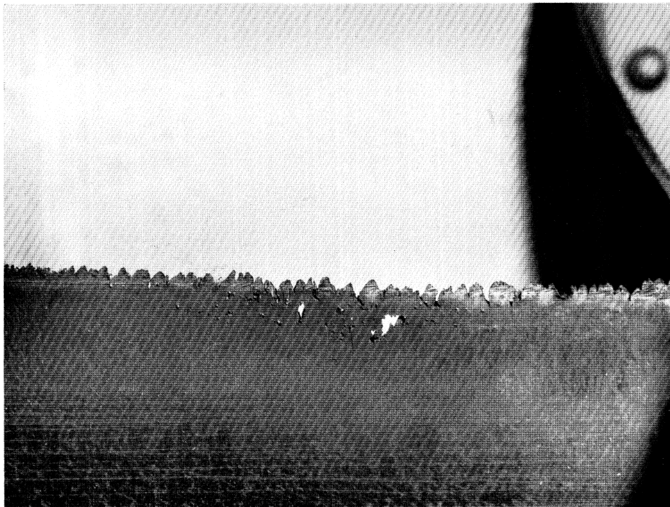
FIGURE 6. Working face of moving blade showing perforation damage caused by water C on figure 5 after 8200 h in service.
