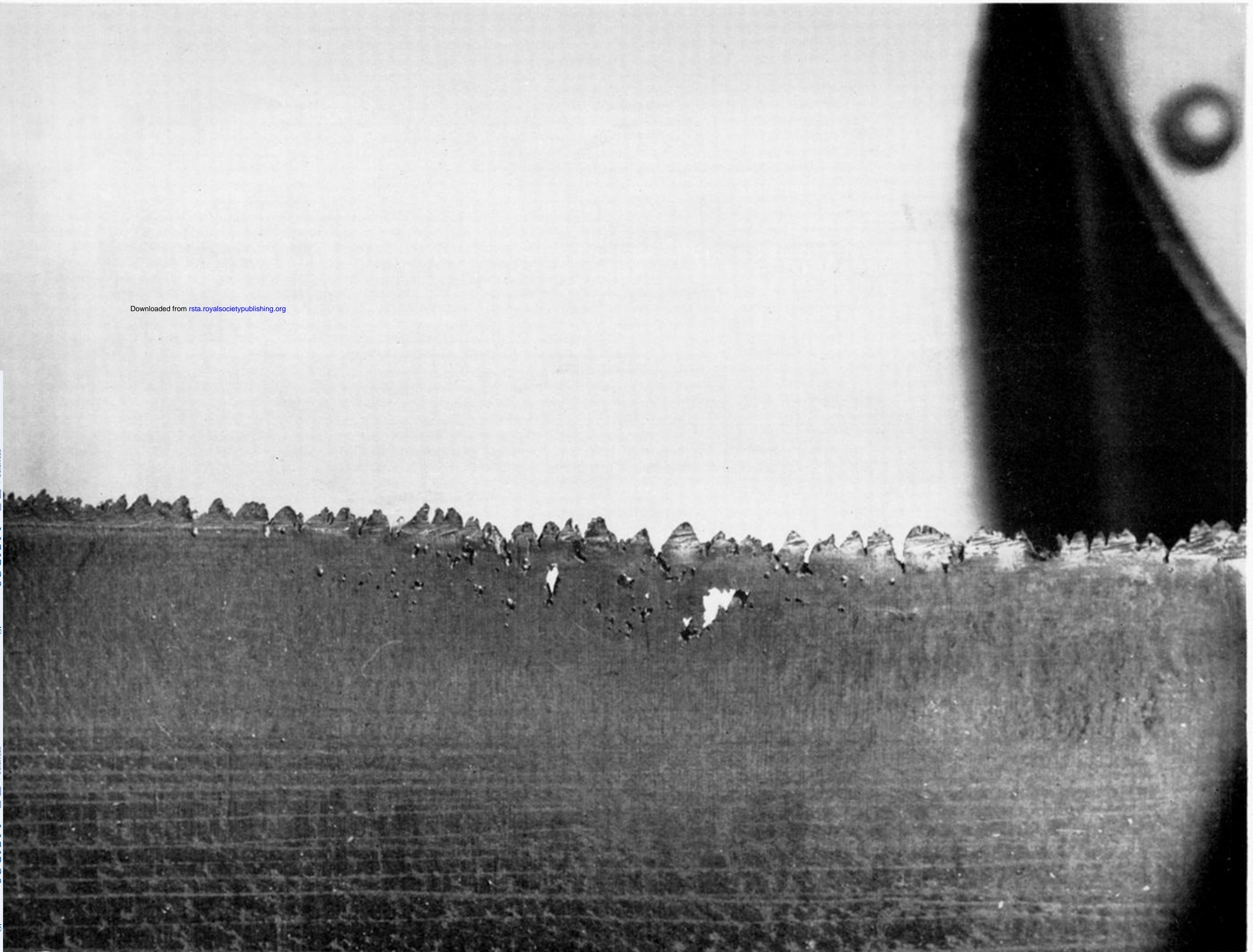
FIGURE 6. Working face of moving blade showing perforation damage caused by water C on figure 5 after 8200 h in service.
