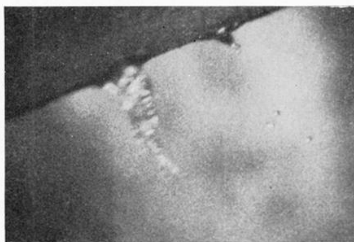
FIGURE 11. Section of ciné film showing water drops stripping from the trailing edge of the centre blade in figure 10. Steam conditions 0.66 Lb./in. 2 (abs.) and 1020 ft./s. (Read downwards, from left to right.)
