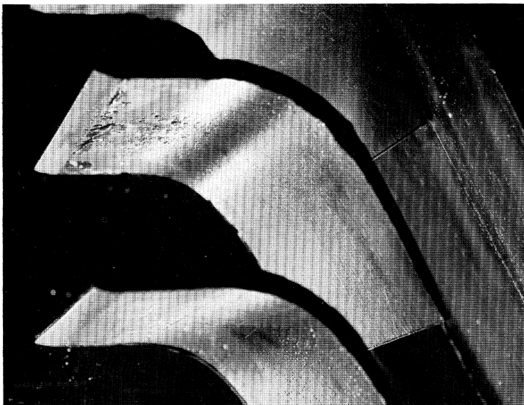
FIGURE 12. Quiescent water puddles in the region of flow separation on the concave surface of a stalled blade.
